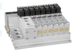
Manifold system with integrated electrical connection including LED indicators, manual override and built-in circuit protection. Valves with connection G 1/4 require 2 stations on the manifold.
