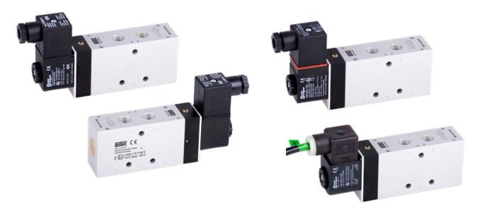
Electrically operated valves conform to equipment category 2 can be used in Zone 1 respectively in Zone 21. For the use in hazardous areas the categry group of the used coil has to be taken into account. The specification of the whole equipment corresponds always to the lowest category of the single components.
